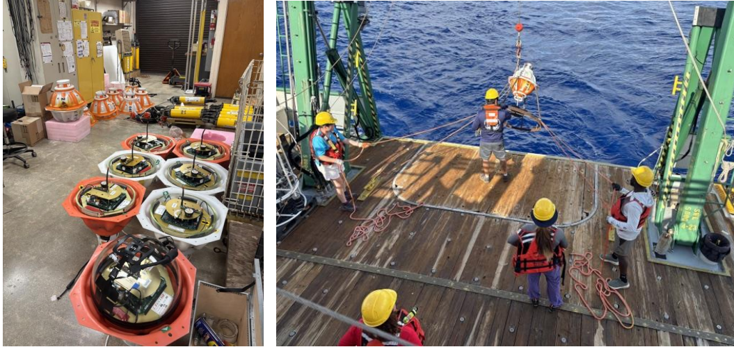
Left: PIES (open half-spheres orange and white) and acoustic releases (yellow cylinders in the back) being refurbished, a very delicate and specialized operation. Right: Deployment of a PIES (Pressure Inverted Echo Sounder)
